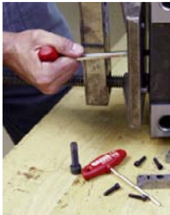
The ball end can be rotated by up to 25° in both clockwise and anti-clockwise direction.
